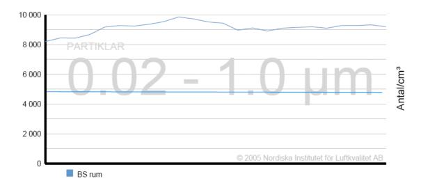
The upper reference graph show high values. The lower graph show result after cleaning. Note the big difference. It is very difficult to clean within this particle spectrum since the particles are so small and the room can already be considered clean. This is a difficult test for the ionizing air cleaner, which it perform very well (Please see reduction test above).
