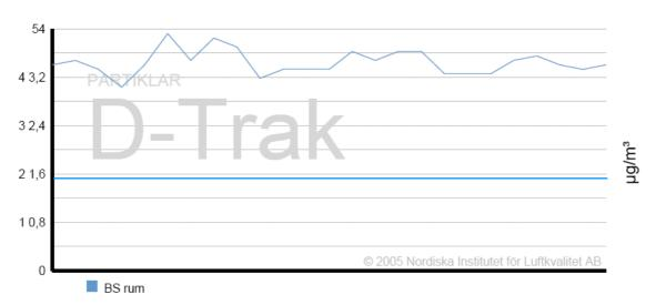
The upper graph shows the reference result that was taken before the reduction test. The graph below shows the average result after 19 minutes of cleaning. As one can see there is a clear improvement within this particle spectrum after cleaning.
