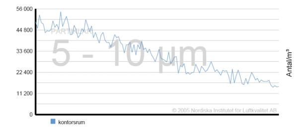
These particles are the first to be seen by the human eye. They sediment fast. We can observe that the ionizer does a good job reducing the number of particles to a level far below the average of good quality air. The reduction of 75% is very good.
