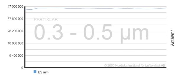
This particle size show that the ionizing air cleaner does not reduce particles, but creates new larger particles of the small particles tested. The reason for this result is that the nano particles tend to agglomerate to larger particles. The bigger particles are however less harmful to humans. The result after cleaning was 40.000.000 particles/m3.
