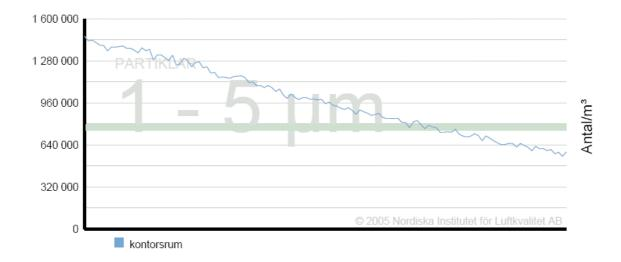
Within this particle spectrum we observe a reduction of 75%, which is good. As these particles can sediment faster than smaller particles they can be more difficult to trap for an air cleaner. The gray line shows an average of normal air in Stockholm. The ionizer continues to show a good result. Within this spectrum you will find bacteria and certain pollen.
